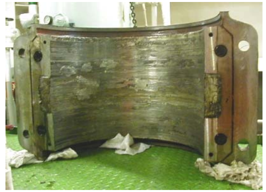
Damaged White Metal Bearing
